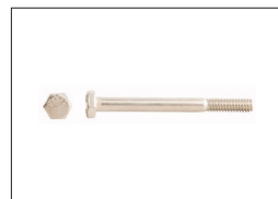
5/16"-18 X 2-1/4" ASTM F593 18-8 STAINLESS STEEL HEX CAP SCREW 4X
