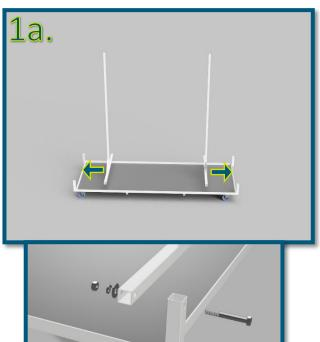
Tighten hardware down on all 4 corners until split lock washer sits flat.
