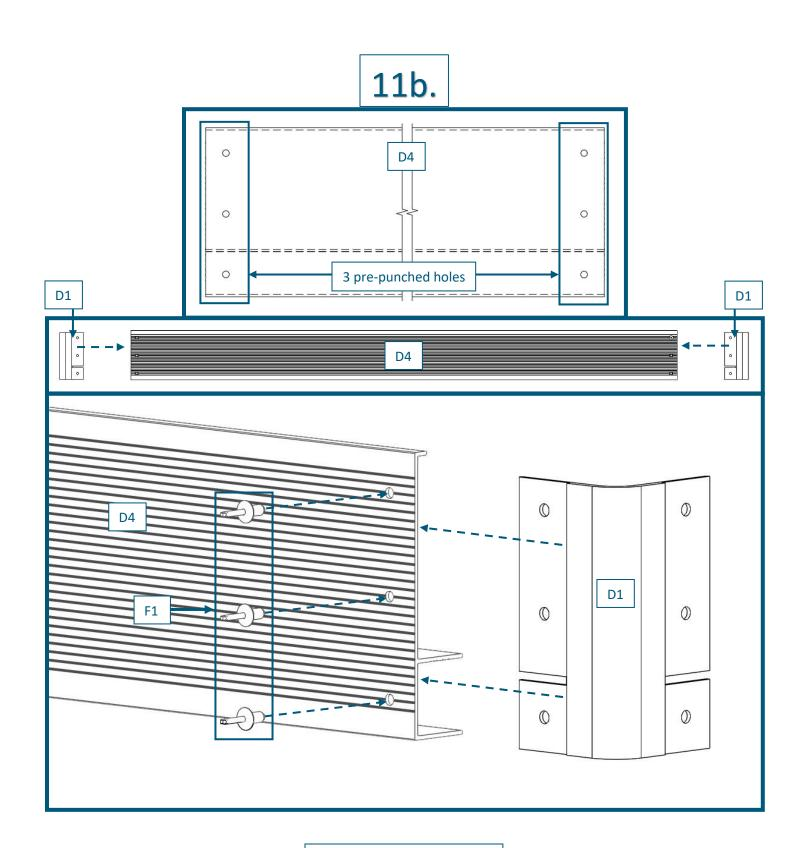
■ If your bench is 5' or wider, install (D4) Bench End Rail w/ (D1) Bench Corners onto end of (D2/D3) Side Rail-side A&B with provided (F1) Pop-Rivets. End Frame will slide into extruded channel of (D4) End Rail, install (F2) Self-tapping screws through top extruded lip into 1" x 1" tubing. Repeat for opposite end. Shown Fig. 11c.
