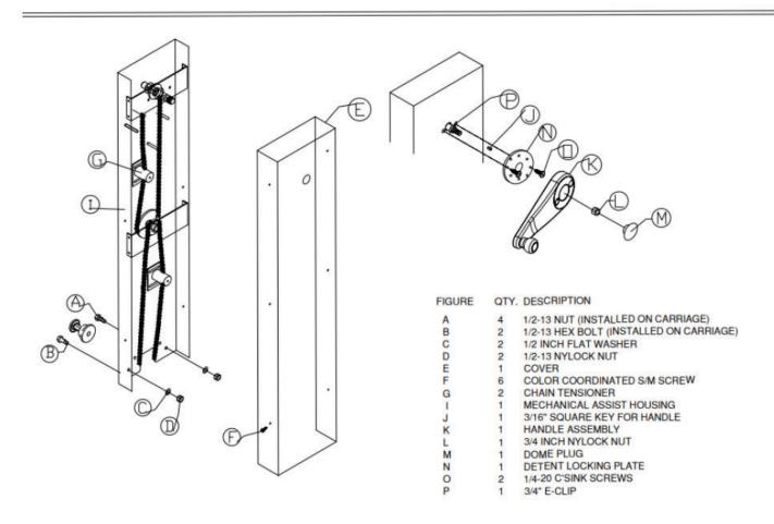
NOTE: OBSERVE THE LOWER CHAIN ROUTING. CHAIN MAY NOT FIT PROPERLY IF ROUTED DIFFERENTLY.
