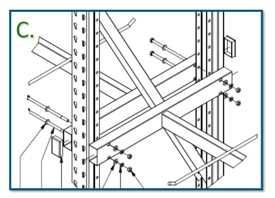
Note: Mallet may be used in this process to seat hardware in place.
